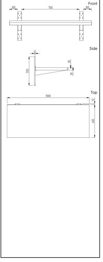
PLUS - Static Preparation 1000 mm Solid Wall Shelf with Brackets
